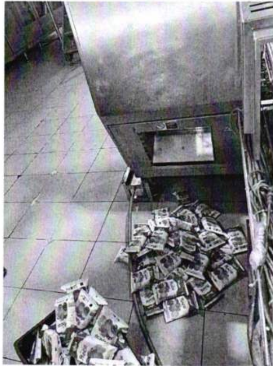
Image 13 Rejected packs discharged at the filler reject chute, upstream of the monitoring point
